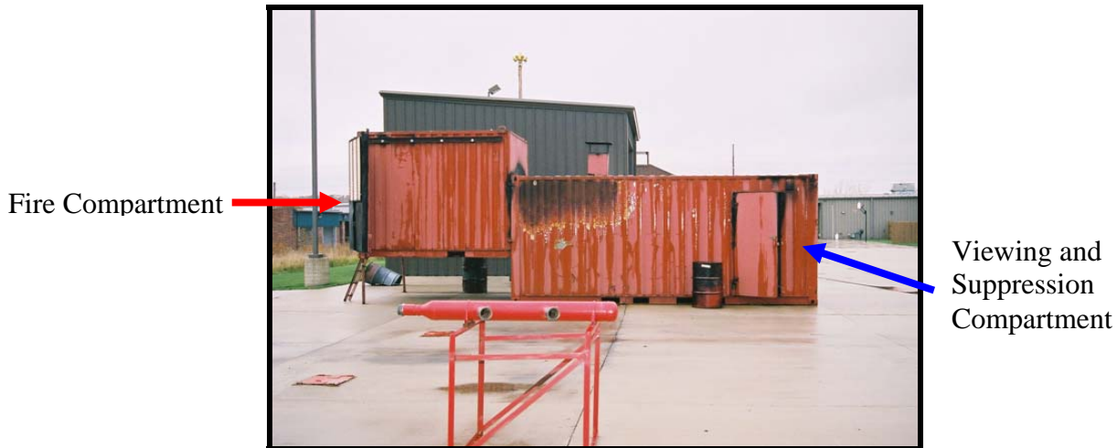
Figure 5: “Flashover” chamber (Photograph of Auburn, Indiana Fire Department Training Facility)
