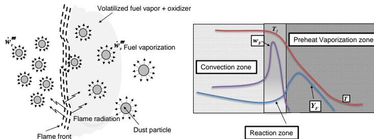
**Figure 1: Schematic illustration of the structure of a dust-oxidizer flame. The fuel vaporization rate is given by  $\dot{w}_v'''$  in units of mass of gaseous fuel vaporized per unit volume per second and the overall reaction rate is given by  $\dot{w}_r'''$**
