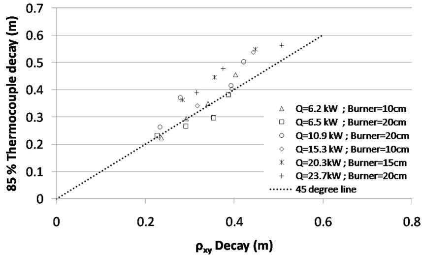
**Figure 9: Plume width measured using a thermocouple tree versus plume width predicted by the decay in the CCV nondimensional cross correlation coefficient.  $f = 10 \text{ kHz}$ ,  $t_T = 10 \text{ s}$ .**
