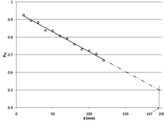
**Figure 5: Nondimensional cross correlation coefficient  $\rho_{xy}$  versus thermocouple separation distance  $d$ , sampling rates 2 kHz,  $t_T$  of 15 s,  $Re = 4200$ . This figure shows the linear decay of  $\rho_{xy}$  with increasing separation distance.**
