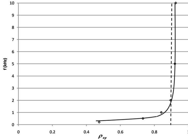
**Figure 7: Sampling frequency  $f$  versus nondimensional cross correlation coefficient  $\rho_{xy}$  for a thermocouple separation distance of 10 mm using a 15-second sampling time. The nondimensional cross correlation coefficient reaches an near asymptotic value at 2 kHz.**
