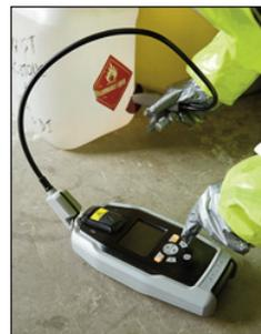
Manufacturer's literature advises that the system is waterproof to one meter submersion, operates in ambient conditions of -20 °C to +40 °C and is rugged as per MIL-STD-810F compliance for drop, shock, and vibration. However, these specifications were not the object of the testing.
