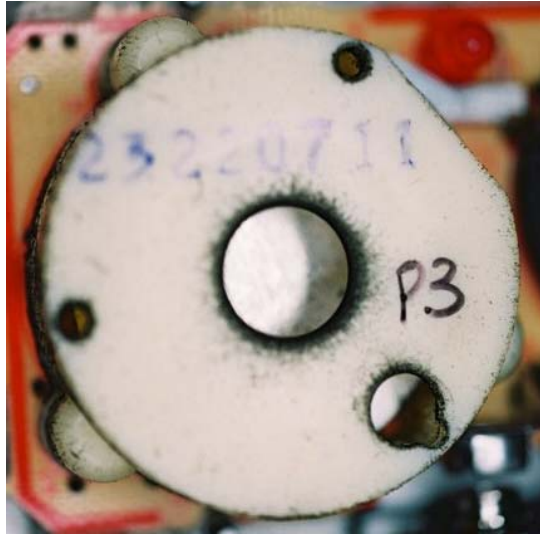
Figure 8 – Acoustic Soot Agglomeration around central and circumferential sound holes of a powered horn disk enclosure.
