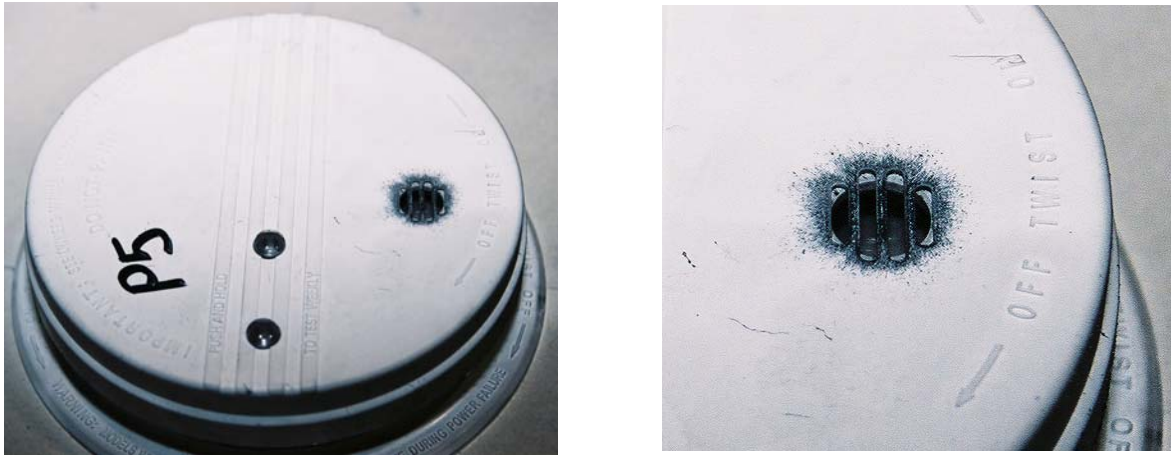
Figures 10 a. and b. – Acoustic Soot Agglomeration around the sound exit grillwork of a Kidde Smoke Alarm
