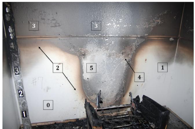
FIG. 1—Photograph from which selected images of visible damage indicators was chosen for use with the DOFD Method.
