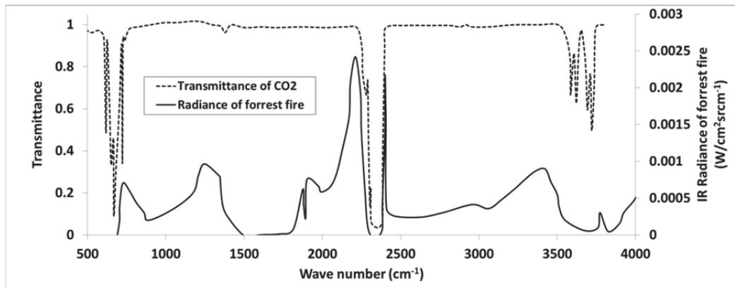
Figure 2: Transmittance of CO<sub>2</sub> versus the emission spectrum of a forest fire.
