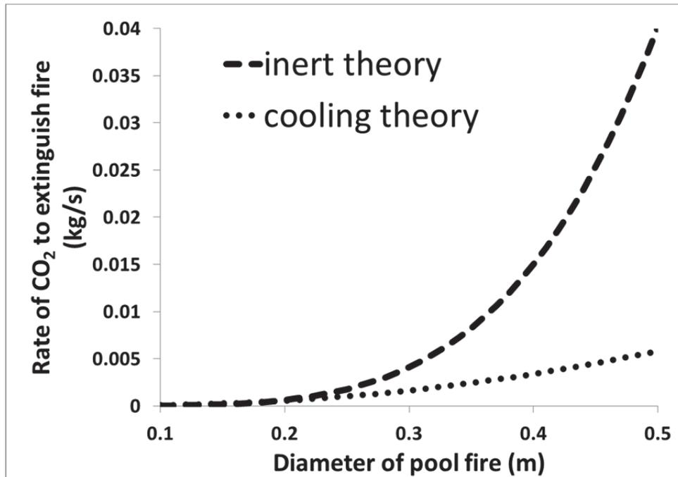
**Figure 4: Comparison of theoretical rates of CO<sub>2</sub> required to extinguish flame for inerting theory vs cooling theory**
