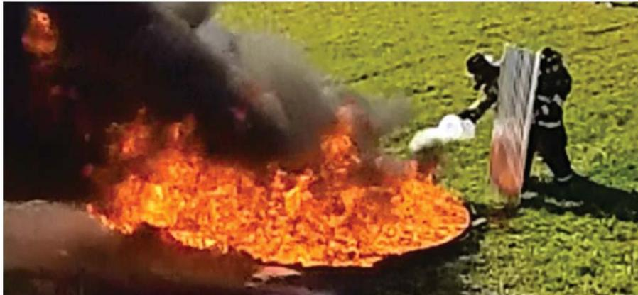
Figure 5: Dry ice being thrown onto 2.44m diameter kerosene fire
