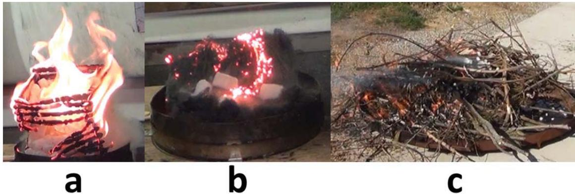
**Figure 8: Dry ice on burning solid fuels. a: Dry ice filled wood crib of popsicle sticks 11cm<sup>2</sup>. b: Dry ice on smoldering steel wool in 17cm diameter steel pan. c: Dry ice on fire of assorted sticks on 122cm diameter steel pan**
