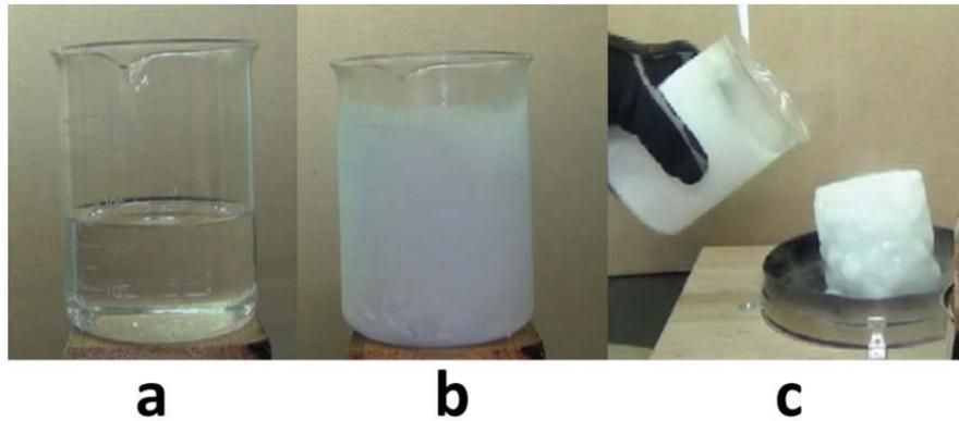
Figure 1: Freezing kerosene with dry ice. a: 250ml of kerosene. b: 500ml of kerosene and dry ice. c: Frozen kerosene/dry ice mixture removed from beaker
