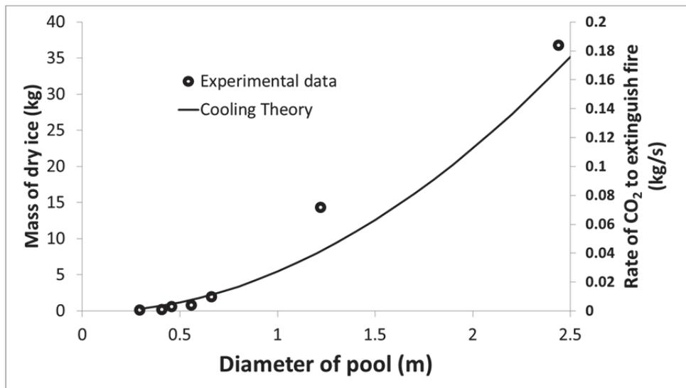
Figure 6: Left axis - Mass of dry ice required versus pool fire diameter. Right axis – Cooling theory CO<sub>2</sub> requirements versus pool fire diameter
