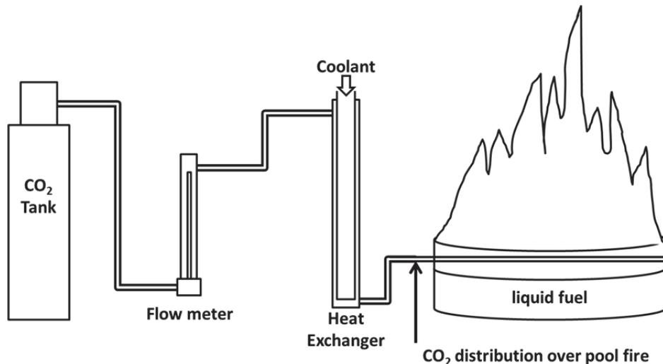
**Figure 3: Diagram of CO<sub>2</sub> temperature experiment**
