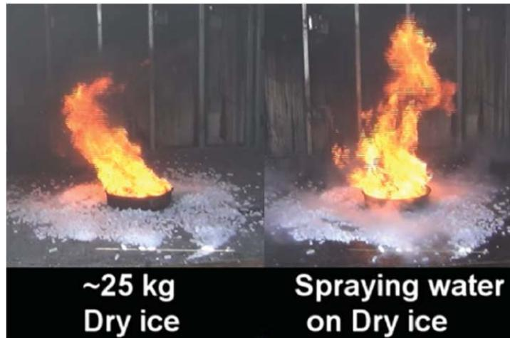
**Figure 7: Dry ice spread around pool fire with and without water being applied onto the dry ice**
