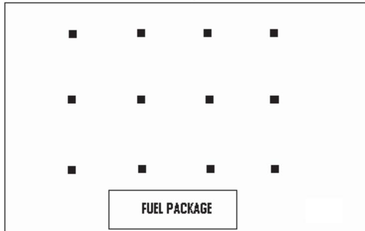
The burn cell for the conical patterns was similar to the one mentioned above, with dimensions being 6'x6'x6'. This cell was also lined with 3/8 inch drywall, with doubled ceilings. The sheet was predrilled with holes for thermocouple probes to be inserted as the rear wall. These were staggered eighteen inches from the sides and bottom, then spaced twelve inches apart horizontally, and spaced six inches vertically, forming three rows of four (Figure 2).
